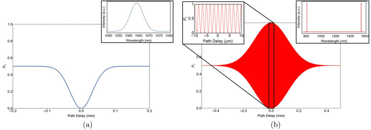
Figure 1. Hong-Ou-Mandel interference patterns for (a) degenerate photon pairs centered at 1064 nm (inset), and (b) frequency-entangled photons with center wavelengths 810 nm and 1550 nm (right inset).
