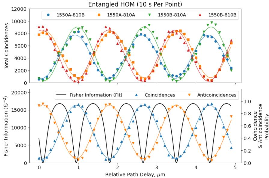
Figure 3. Characterization results for the nondegenerate frequency-entangled interferometer. (Top) Coincidences (blue and green) and anticoincidences (orange and red) measured as a function of relative path delay. (Bottom) Net coincidence and anticoincidence probabilities (blue and orange), along with extracted Fisher information. As expected, Fisher information is maximized when the slope is steepest.
