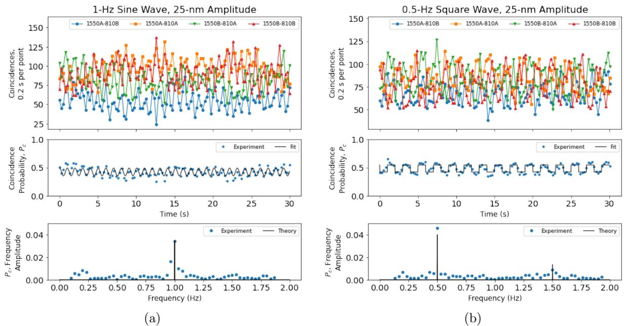
Figure 5. Measurement of 25-nm vibrations using frequency entangled interferometry for (a) a 1-Hz sine wave, and (b) a 0.5-Hz square wave. (Top) Raw coincidences (blue and green) and anticoincidences (orange and red) measured during 30 second scan. (Middle)  $P_c$  calculated from both coincidences and anticoincidences during the scan. (Bottom) Fourier transform of  $P_c$  used to extract the vibrational modes.
