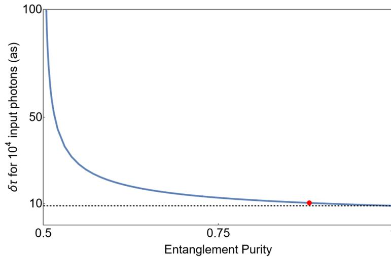
Figure 4. Relationship between entanglement purity and measurement resolution ( $\delta\tau$ ) for  $10^4$  detected photon pairs, approaching the quantum Cramér-Rao bound as purity increases. Our current result of 10.3 as resolution (red circle) represents an 88% saturation of the bound.
